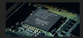
DIGIC DV II includes a hybrid noise reduction system that uses inter-frame and intra-frame prediction to ensure virtually noise-free video output. This, along with a new gamma system, reduces noise in monotone and shadow areas to give you crystal clear high definition images.
